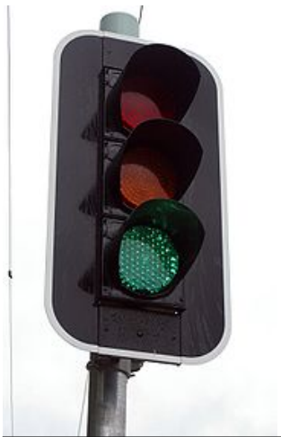
LED traffic lights use 80 - 90% less electricity and have a longer life than regular traffic signals that use incandescent bulbs.
